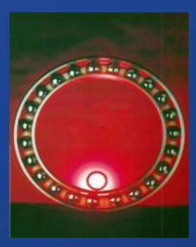
There are three types of thin-section bearings: deep groove bearings, four-point contact bearings, and angular contact bearings. Compared with standard-section ball bearings all three bearing types offer advantages in reduced space requirements and low cost. These bearings are used primarily where shaft location is the major requirement.
